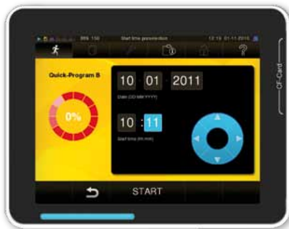
Time pre-selection for automatic autoclave start
